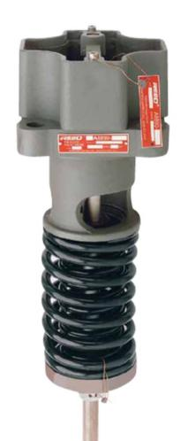
Rego's A8890 Series Pressure Relief Valve is a 304 Stainless Steel low profile, heavyduty, PRD with industry leading flow rates. It's dual epoxy coated springs offer extended wear and is designed to keep operating should one of the springs fail. Other engineered features, include an intermediate spring guide for positive reseating, a robust stem, easy access mount fasteners and its ability to mitigate escaping vapor (rather than product) into the atmosphere.
