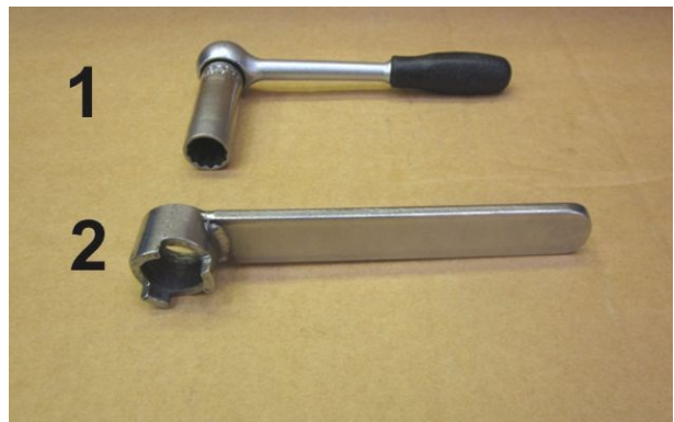
Step 8. Select the tools required to remove the poppet assembly: 1. 1/2" (13mm) socket wrench. 2. Spring pad locking tool, part no. 400/7495.
