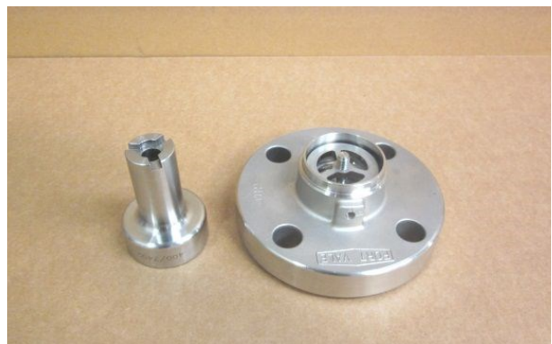
Step 12. Select the spring pad assembly tool, part no. 400/7492. The tool lets you disassemble the poppet, spring and spring pad from the valve body.
