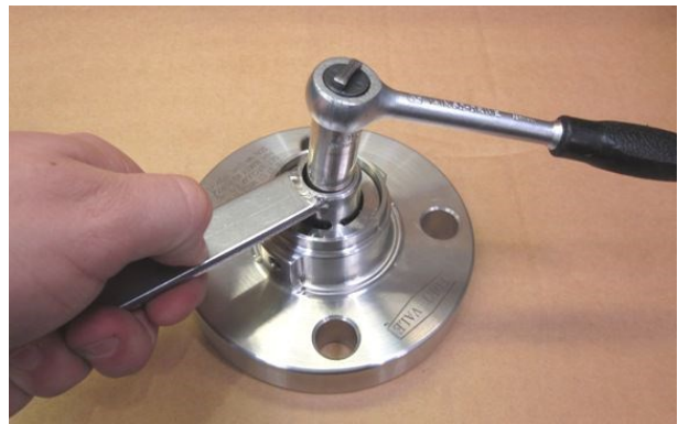
Step 10. Hold the locking tool to prevent the spring pad from turning. Unscrew the 5/16" UNF nut with the socket wrench.
